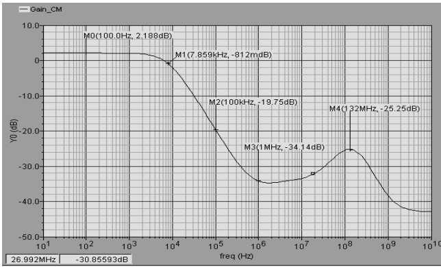
Fig. 7. Simulated results of the gain for a common mode signal at the input.
